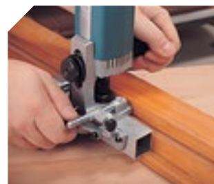
Slotting a window, lock side.
