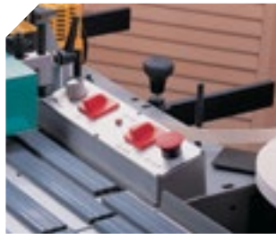
Safety control (STOP). Electronic temperature control.
