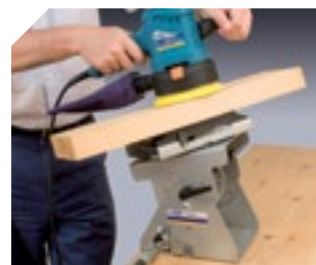
Adjustable tilting and swivelling support.
