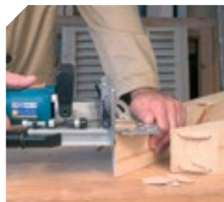
Stronger joints with No. 6 splines.
