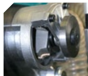
Separate copier from the bit.
