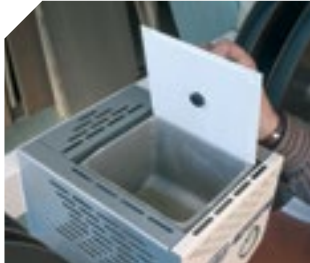
Easy access glue tank on top. The glue application system includes an easy, non-stick silicon roller.
