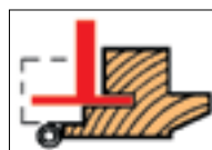
Slotting a window, hinges side.
