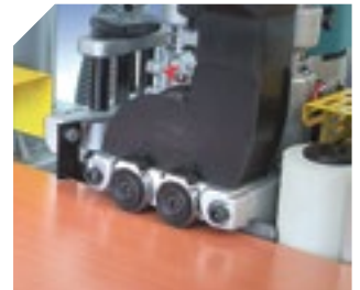
Simultaneous top and bottom trimming, with radius or 10^\circ chanfer. Flat scrappers after the trimming unit.
