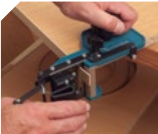
Cutting on both sides on straight panels.
