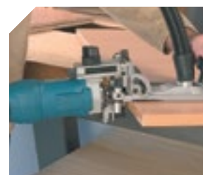
Trimming the edge with the straight bit.
