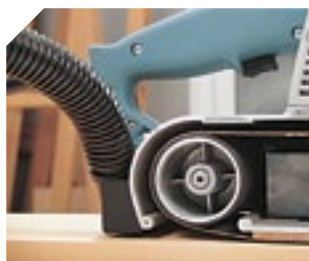
External dust collector connection on model LB31E.
