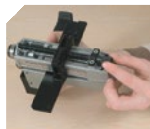
Micrometric regulation of the cutting width.
