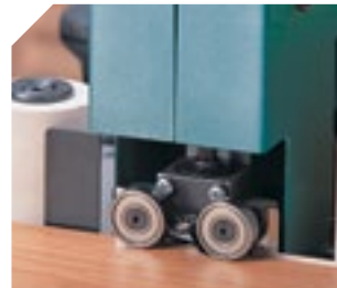
Power trimming unit: trimming both sides simultaneously.
