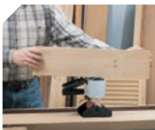
Gluing with the upper roller.
