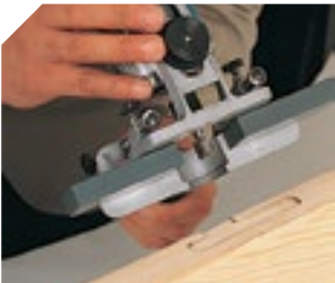
Placing hinges with the ZB93 head.
