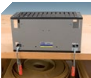
Small piece clamped on divisible suction plate.
