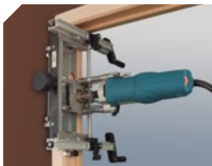
Making the upper recess on the frame.
