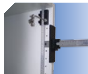
Drilling for placing invisible hinges.
