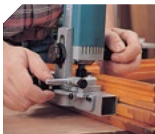
Slotting a window, flashing side.
