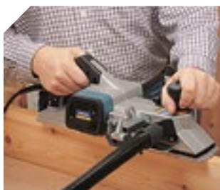
Dust collector connection.
