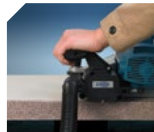
Working on solid surface material (i.e. Corian®).
